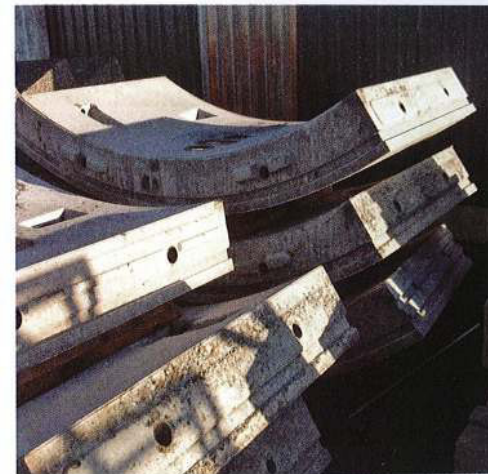
Figure 1: AACM tunnel ring segments precast by Shay Murtagh Precast with steel fibres in the mix design.
