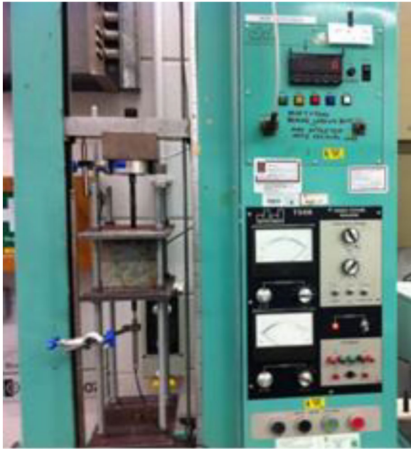
FIGURE 4 Pull-out test arrangement [Color figure can be viewed at wileyonlinelibrary.com ]
